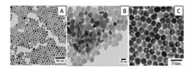
Fig. 1: Silver (A) and Copper (B, C) NPs of different shapes obtained by chemical synthesis process developed in MONARIS laboratory
